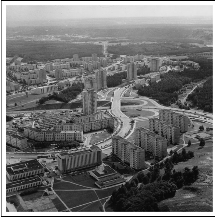
Figure 5. Lazdynai residential district (Vilnius, Lithuania; 1967). High-density panel apartment buildings surround community services in the housing estate. Pathways connect important origins and destinations and bus transport.
